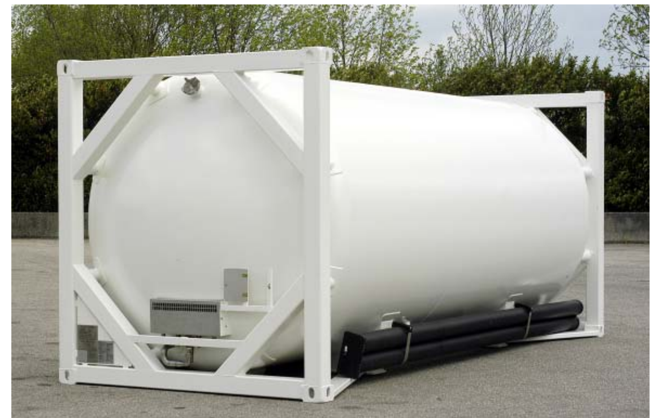
All ISO tank containers are vacuum multi-laminar super insulated.
