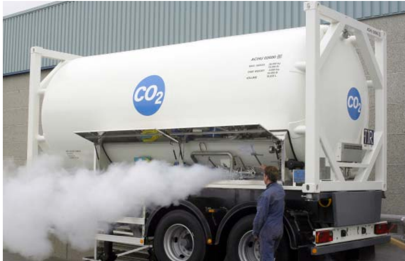
Machinery compartment with transfer pump on one side and lockable hose boxes with transfer hoses mounted on opposite side.
